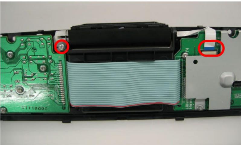
**(18) Logic board ass'y wiring**
